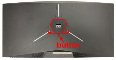
2. Remove the original screws from the opening in the back of the monitor. Please save these screws for Step 4.
