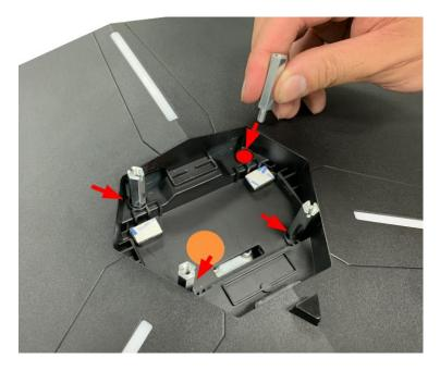
4. Install the wall mount plate on top of the standoffs and secure the plate by tightening 4 wall mount screws onto the plate.
