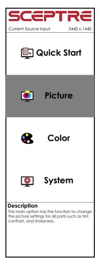
When you press the **M** button on the monitor, the OSD screen will appear. Select each of the functions with the  $\blacktriangle$  or  $\triangledown$  buttons. Use the **M** button again to enter each of the function or when you are in the function already, use the **M** button to select the option you want to adjust. Use the  $\blacktriangle$  or  $\triangledown$  buttons to adjust each option's values. When you want to exit press the **E** button.
