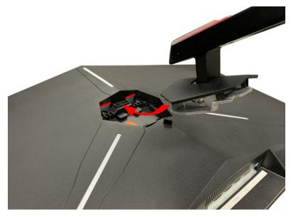
6. Once the back plate's top end goes in push down on the bottom end to secure the stand into the monitor.
